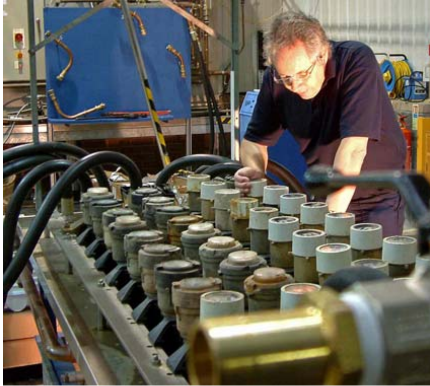
Positive Displacement Meters Under Test
